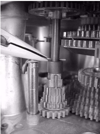
Remove cotter pin above spacer
