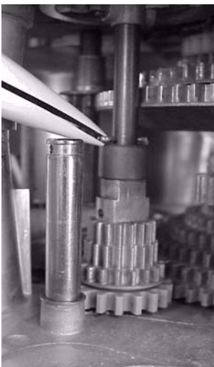
Lower spacer, re-install cotter pin
